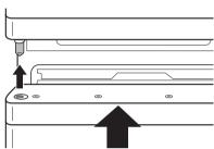
Place the lower door bearing with the bearing pivot in the lower left of the door and fasten.
